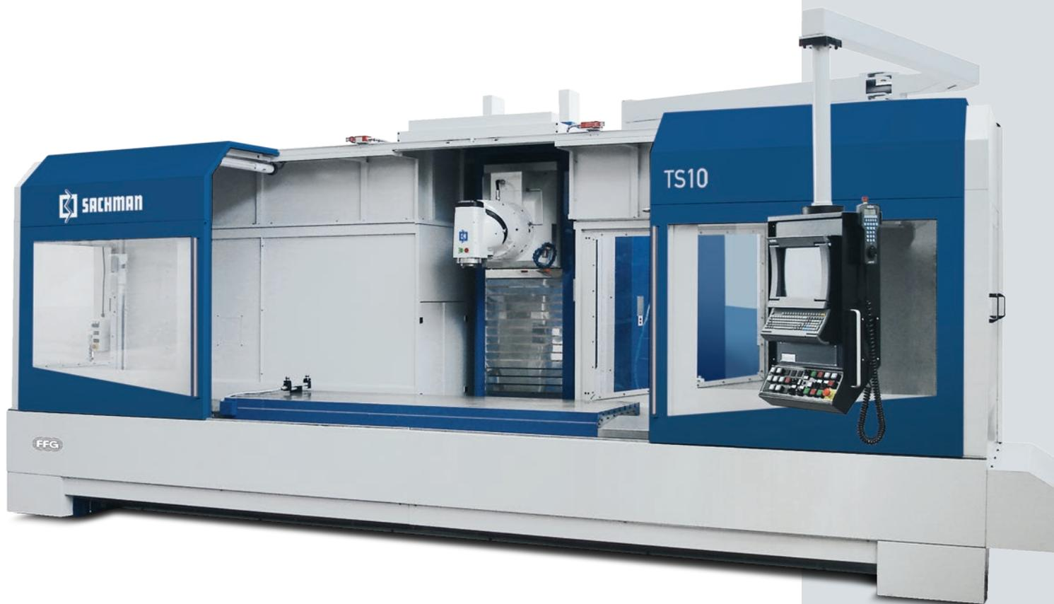
**A**s all products of T and TRT lines, TS10 is characterized by a technical solution, which has been used for years and constantly improved by Sachman: the transversal movement of the column and the absence of the slide. This solution ensures geometric accuracy and great chip removal capacity regardless of the position of the transversal axis, as well as an excellent visibility of work area and accessibility to the spindle.
