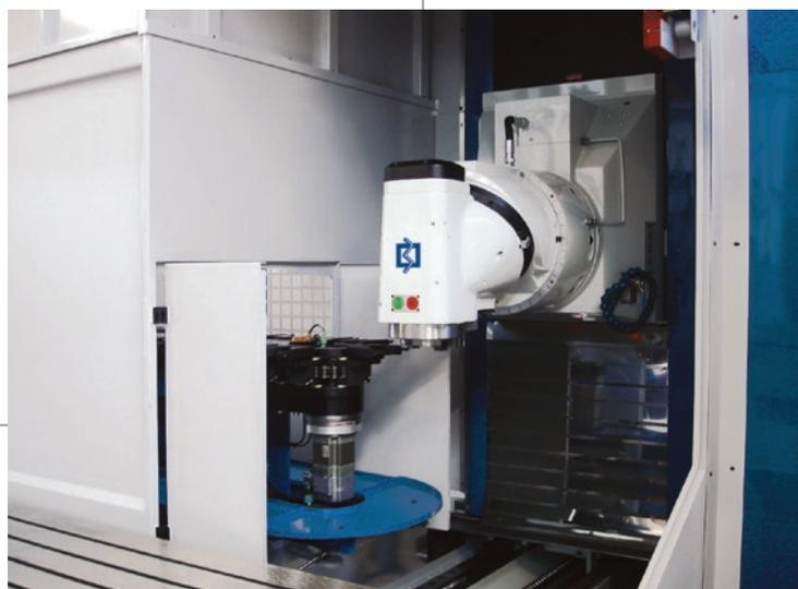
**T** S10 utilizes a roto-translating chain tool magazine with either 24, 40 or 48 (optional) pockets. The exchange occurs when the column is totally withdrawn in order not to cause any sort of interference with the working area.
