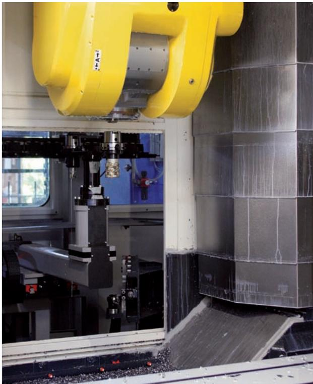
Tarkus can be equipped with a chain-type magazine that can hold 32 to 64 tools; other magazines are available with static configurations for up to 180 tools.
