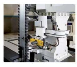
Chain-type tool magazine with 40/60 positions ISO50/HSK-A-100
