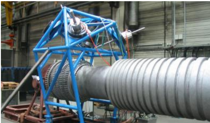
Mobile Milling unit for maintenance of turbine drive shafts (METROM / IWU)
