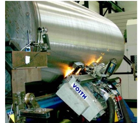
Mobile Grinding unit for maintenance of rolls for paper drying (Voith Paper Services / IWU)
